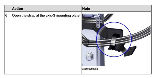
Removing the protection hose (protection type Foundry Plus)
